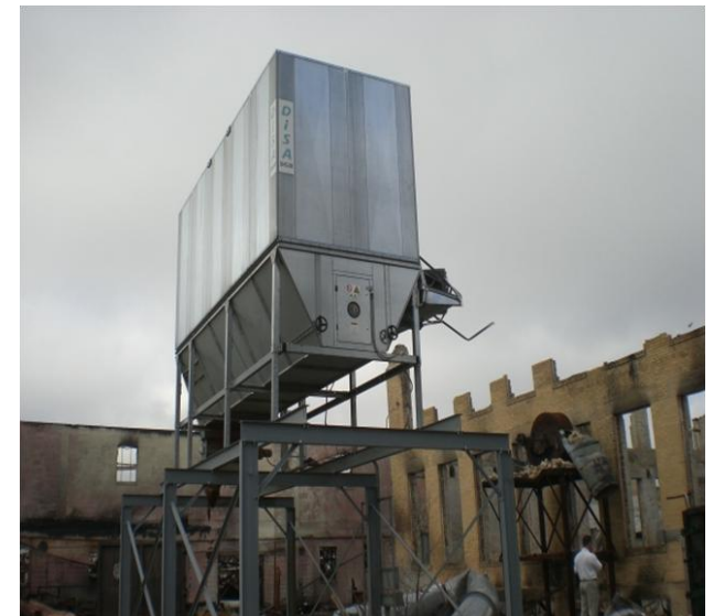
Only thing left intact of the plant was the dust collector
