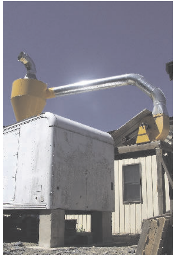
Return to come — Currently the new dust collection system at J&J Custom Woodwork in Stroudsburg, Pa., empties into a trailer outside. Plans call for finishing the system with a return air line so heating and air conditioning in the shop will function properly.
